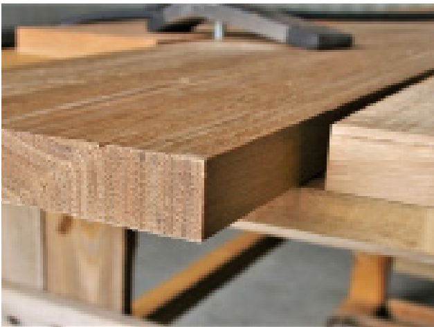
Clean corner on exit side with no “blowout”!
