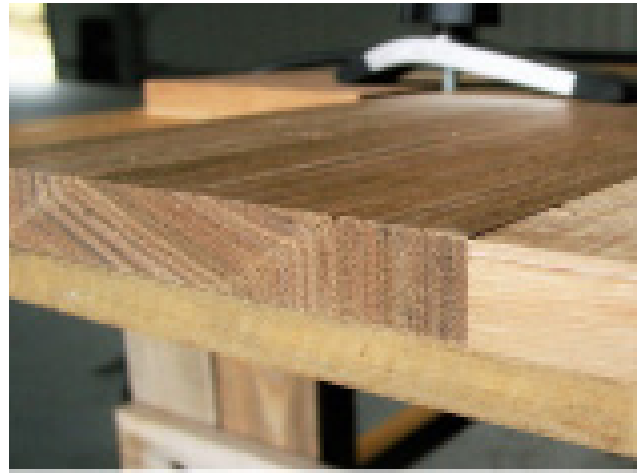
End Grain Routing with support piece
