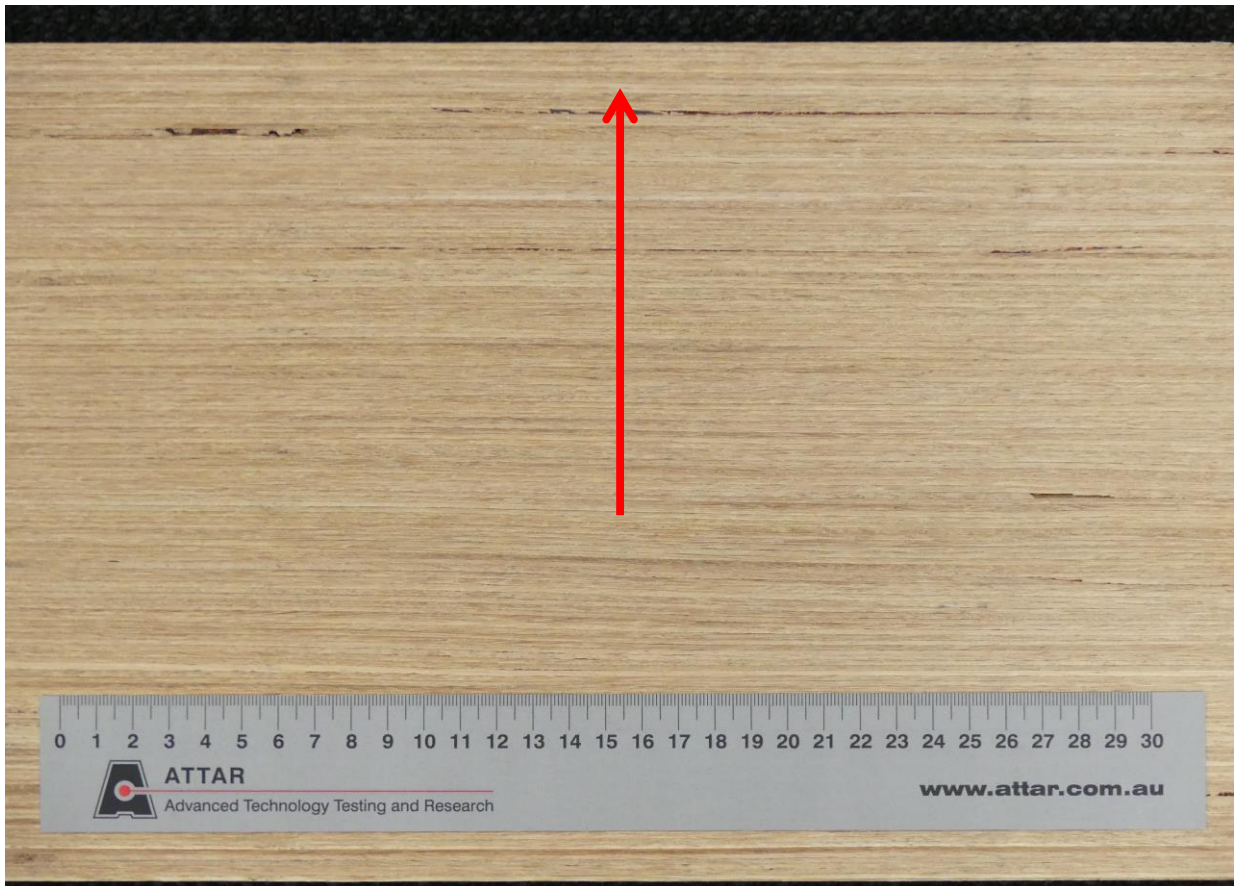
Figure 1: Stair Tread Blackbutt Arrow indicates direction of testing
